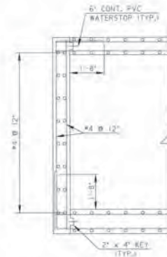
SECTION AT END OF TUNNEL SCALE: 1/2" = 1'-0"
