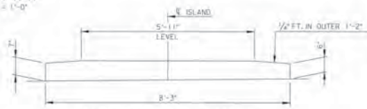
6" RAISED MEDIAN DETAILS ISLAND 1 (ONLY) SCALE: 3/8" = 1'-0"
